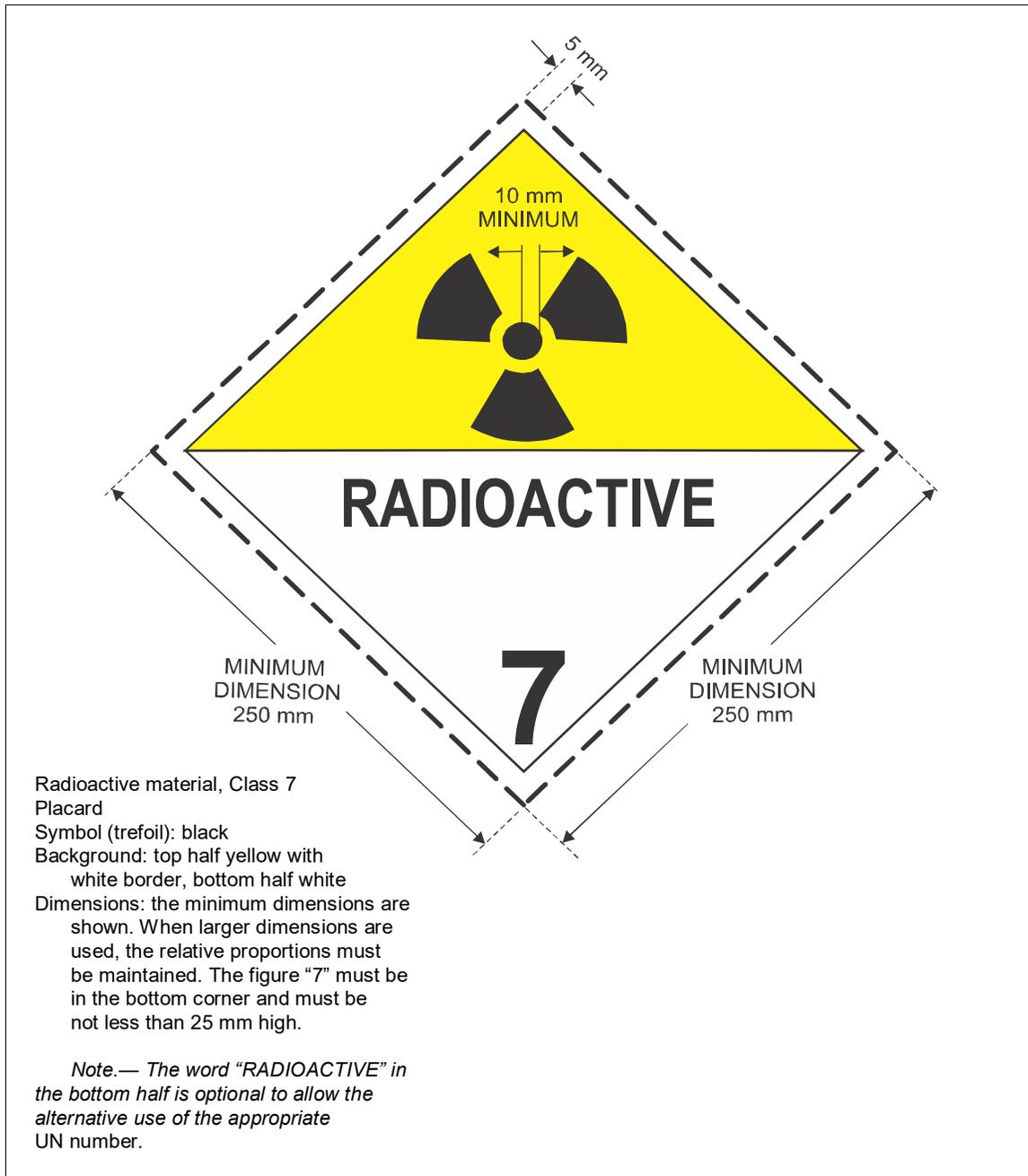
Figure 5-30. Radioactive material, Class 7, placard for large freight containers
