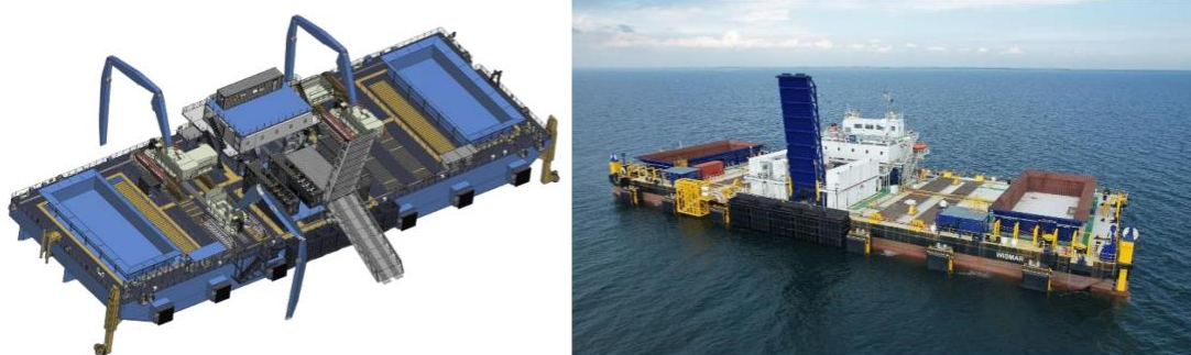
Figur 6: Protection Layer Ponton
