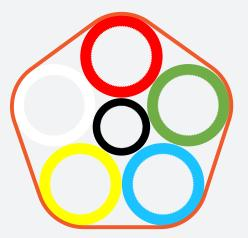
Höhle microducts are designed for long term protection of fiber optical cables. Direct Bury (DB) type of microducts are thick wall products that attain their mechanical robustness and functional performance through their intrinsic thick walls and need no further protection at underground installations.
